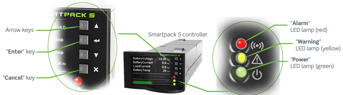
Figure 6. Smartpack S controller's front keys and indicators
